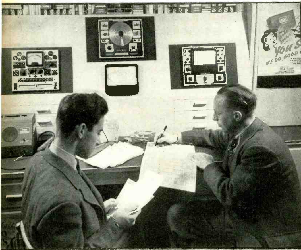
Dealer and assistant in typical job-posting chore. Mark-up of job bills with the right gross margin percent is as important as "mock up" of shop with proper modern test equipment for variety of radio problems. Arrangement of tube checker, sig. gen., v.o.m., sig. tracer, meter is trimmed for 1-man operation. Clock is missing. (Photo courtesy Dale Distributing Co., N. Y.)
