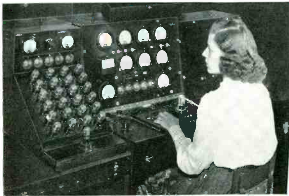
This standardized Hytron production tester is composed of three units: preheater, characteristics tester, noise tester. To permit a better view of the equipment, only one of three operators is shown.
