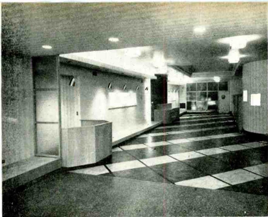
“Basic” display fixtures include built-in low platforms (left) and kidney-shaped counter (middle background)—see plans opposite. Note shadow box lighted with indirect fluorescent and incandescent stem drop fixtures. Floor pattern is intended to make it unconsciously easier for people to walk further into store. Along right wall are individual customer-sales offices; at rear, behind glass wall are the radio servicing department and the shipping room. Enclosure in left foreground is for receptionist and cashier. Out of picture, at right foreground are the stairs and the elevator leading to mezzanine Home Center sales room, where dealer will concentrate major kitchen and home laundry appliance displays, plus smaller tie-in appliances. Comparatively narrow store gets widening effect through well placed lighting and pastel colored walls.
