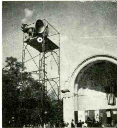
A multi-unit Operadio exponential horn provides high volume to overcome extreme extraneous ground noise
